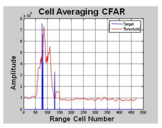
Figure 6 The above figure shows that Cell Averaging CFAR will not work for Range-Spread targets. Here in case of high HRRP's, the threshold is contributing to the target and therefore the target is getting masked.
