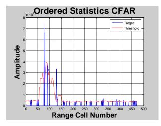
Figure 8 Response of Ordered Statistics CFAR for Range Spread Targets
