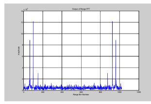
Figure 5 FFT of the extracted Beat Frequencies for 3 targets. As evident from the figure, the filter number which gives the peak response corresponds to the instantaneous range of that particular target. For real signal, the FFT spectrum is two-sided.
