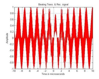
Figure 3 Output of the Mixer after beating Transmitted & Received Signals
