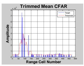
Figure 7 Response of Trimmed Mean CFAR for Range Spread Targets
