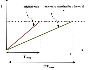
Figure 2 How the effect of Stretch Processing lowers the sampling frequency.
