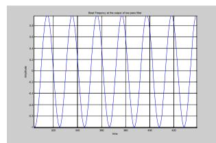
Figure 4 Beat Frequency extracted after Band Pass Filtering. For a single target this is a single frequency sinusoid.
