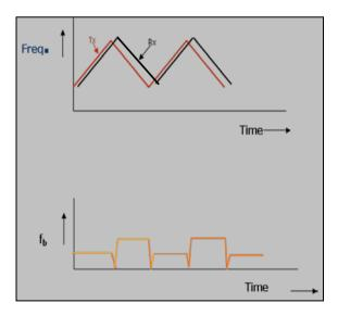
Figure 1 Beating Transmit & Received waveform of targets having a Doppler velocity.
